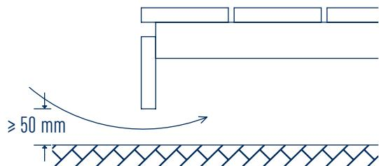
If the side of the terrace is closed with a cover board, a ventilation opening of > 20 mm (continuous) must be maintained for ventilation of the terrace construction. The cover board should not touch the ground.
