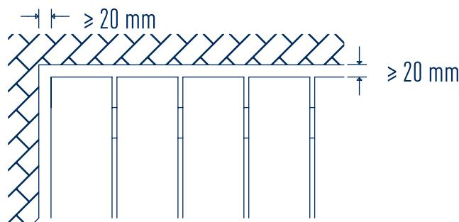
When connecting the terrace to the adjacent building, a distance of > 20 mm must be observed so that the joints cannot close either through dirt or changes to the planks. The unhindered drainage on and beneath the terrace must be permanently guaranteed.
