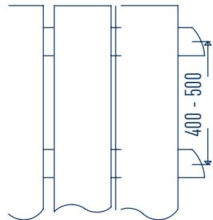
The joint distance for plank widths 90 - 120 mm should be at least 7 mm or 6% of the plank width!
