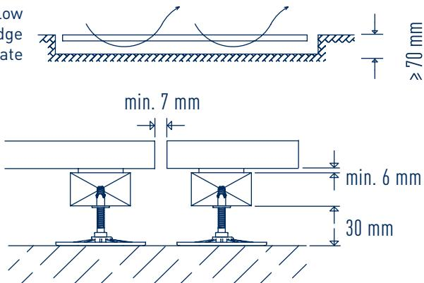
The butt joint should never be installed on the substructure and with a distance of at least 7 mm!
